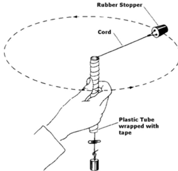
Fig. 4: Centripetal force measured by hanging weights ( $m$ ) to a rotating object ( $M$ ).
